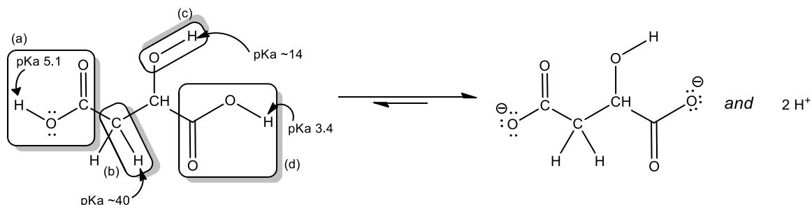
Figure 8.2. The dissociation of malic acid into ions. Hydrogens (a) and (d) are lost as protons . De-protonation (i.e. loss of a proton) does not occur for hydrogens (b) and (c).
