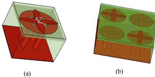
Figure 1. CAD models of unit cells for (a) unmodulated and (b) modulated structures. (In both cases the upper metal plane is removed for revealing the interior).
