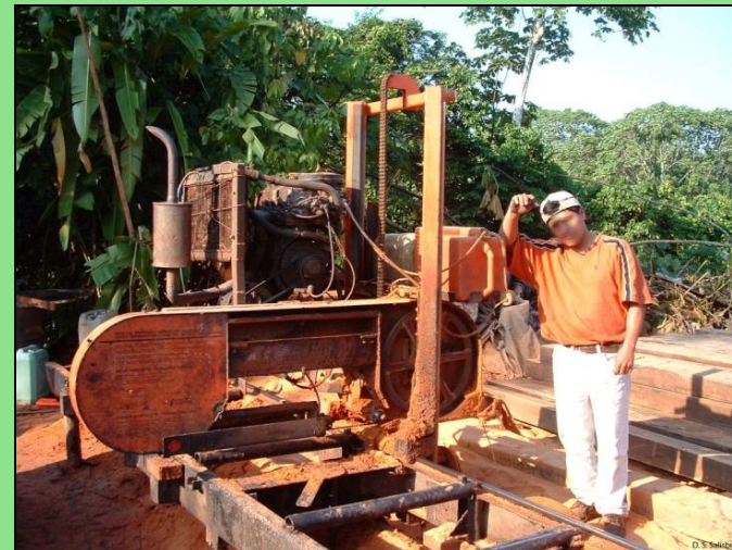
Figure 5: A limpiadora , mobile sawmill, used to refine illegally sawn planks of high value hardwoods
